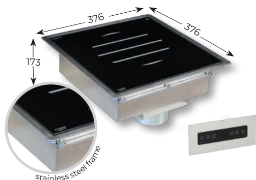
Product cut-out dimensions: 352 x 352 mm Control panel cut-out dimensions: 198 x 68 mm
