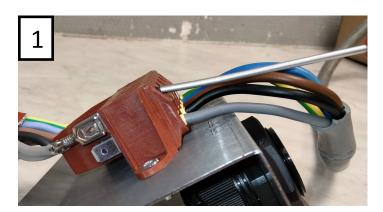
**2** / Then lift the screwdriver to allow the lowering of the spring-loaded jaw of the terminal block contact.
